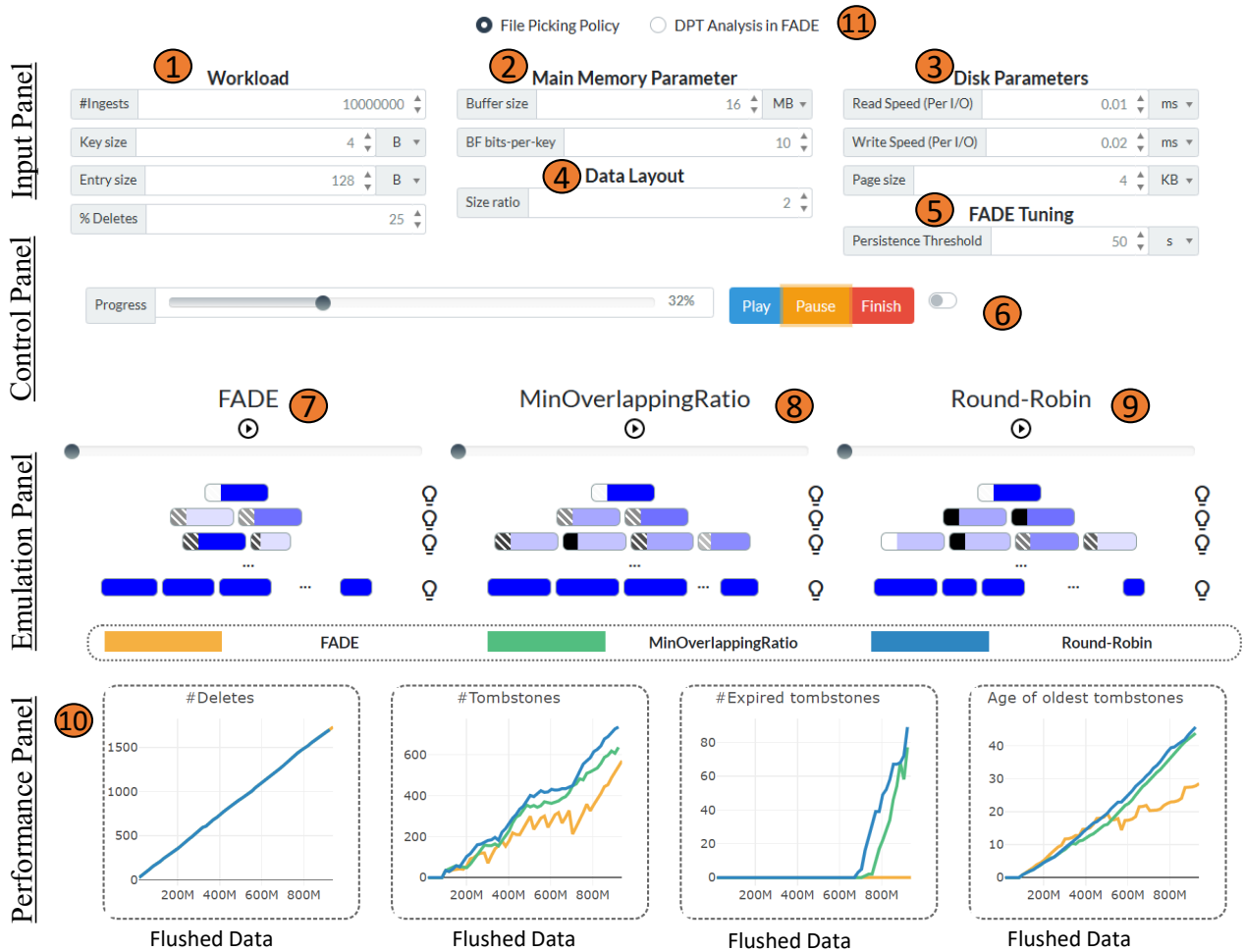
Figure 2: The Acheron UI visualizes the life cycle of tombstones under different compaction policies.
